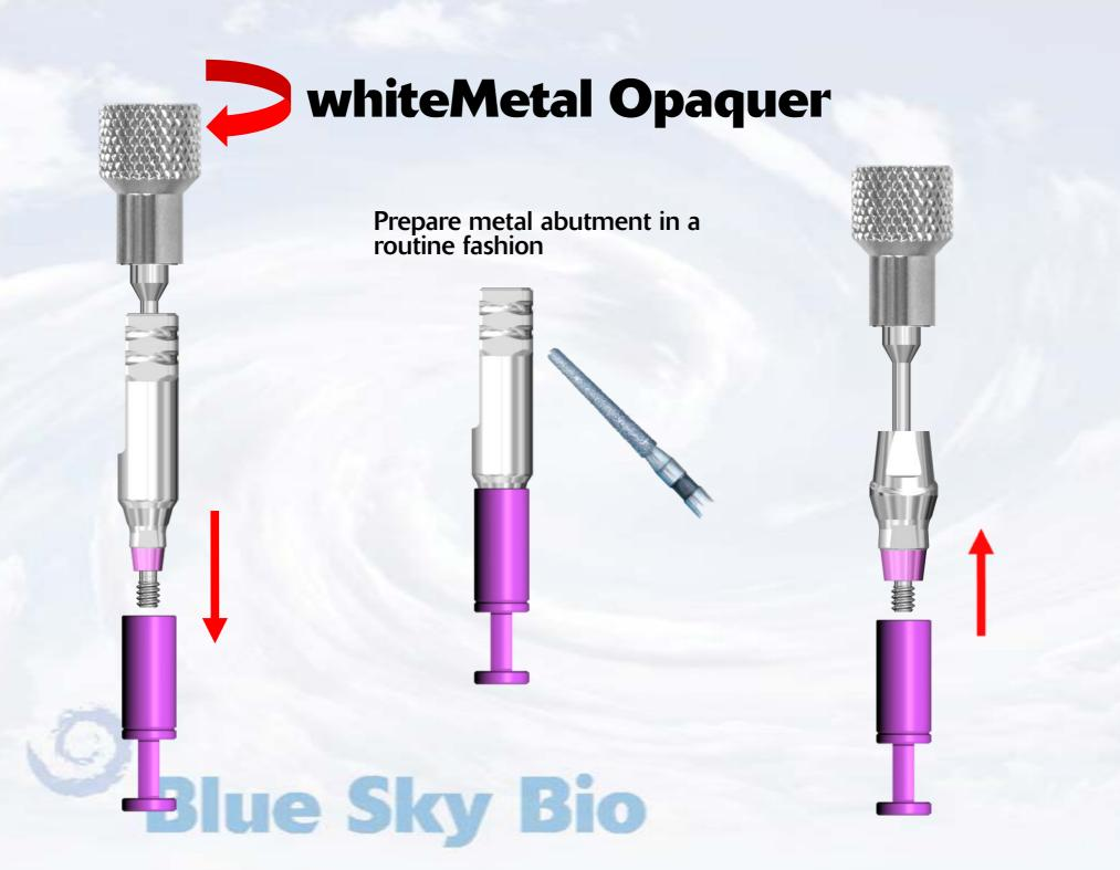
Sandblast the area of the metal abutment to be covered by whiteMetal. Do not sandblast areas that will not be covered by the final restoration. Apply one coat of liquid whiteMetal bonding agent to the surface that will be coated with whiteMetal Opaquer.
